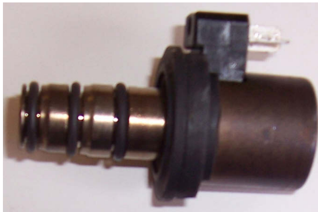
Fig. 18. A macroscale photograph of a solenoid valve belonging to (b) case (partially failed but still run for 24 h).
