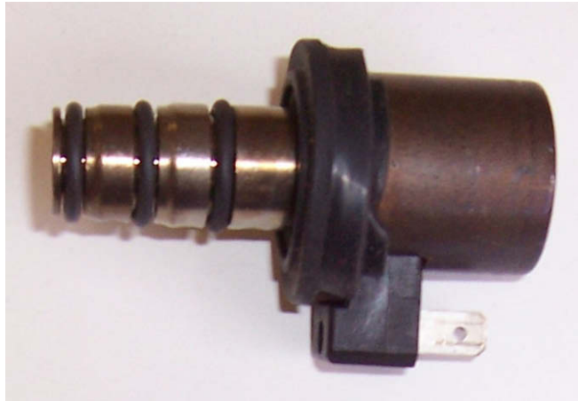
Fig. 17. A macroscale photograph of a SV belonging to (a) case (the solenoid valve was run for 24 h without failure).
